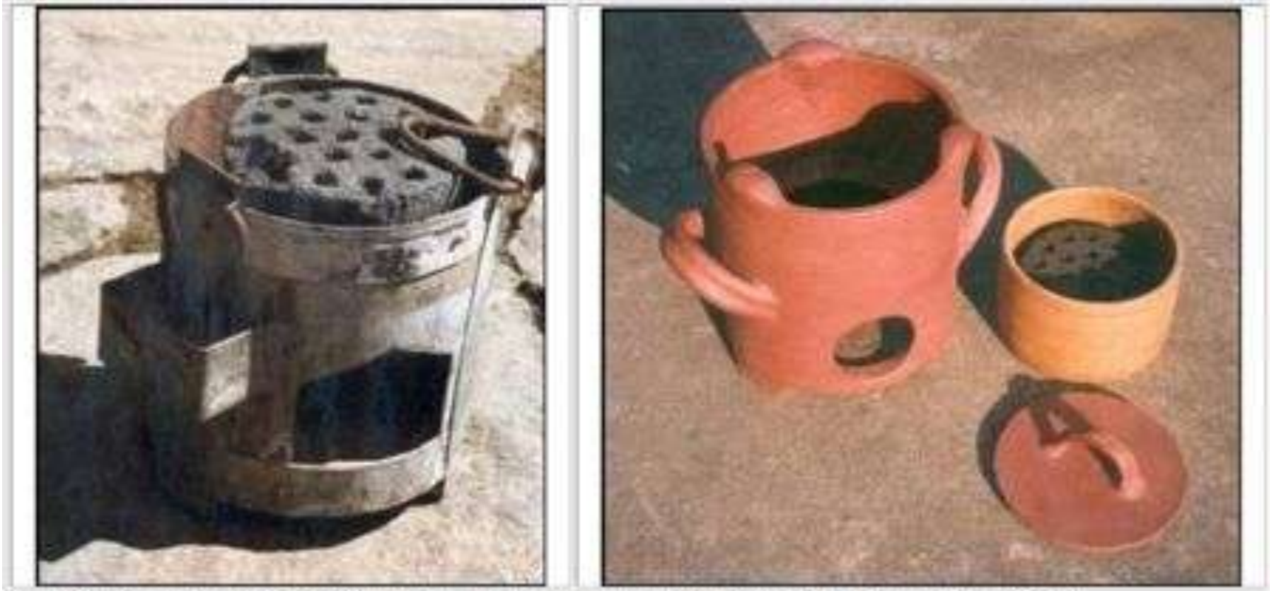
Briquette Stove from which the insulation has been removed (left) and Baked Clay Stove (Right)
